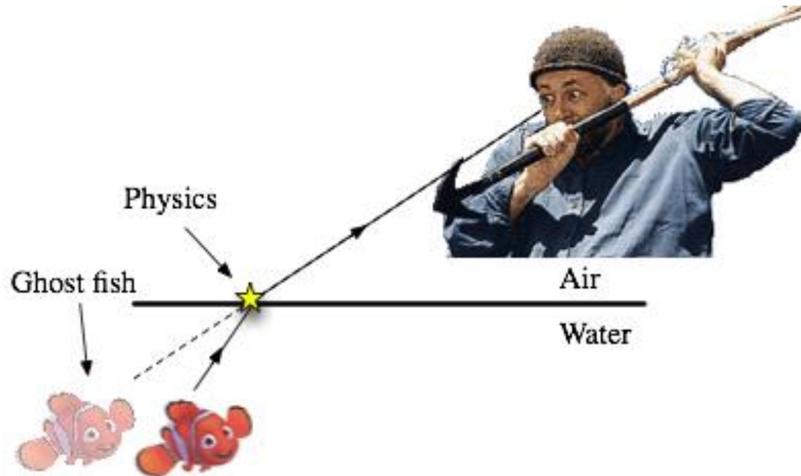
The cause of this is due to the fact that light **BENDS** when it reaches a new medium. The object is **NOT** directly in a straight line path, but rather it's image appears that way. The actual object is on either side of the image you are viewing.
